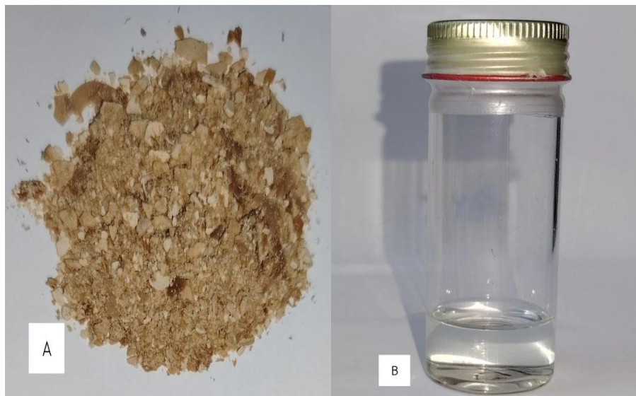
Figure 4. Dried Biomass of C. parapsilosis (A) and Yeast Lipids Extracted with Hexane as a Solvent (B).
