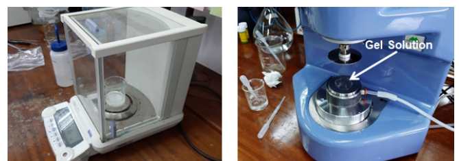
Figure 1. Left: Gel Preparation, Right: Experimental Set up for Rheological Measurements.
