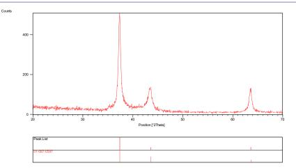
Figure 3. XRD Pattern of As-synthesized Silver Nanoparticles.
