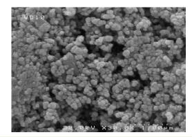
Figure 2. FESEM Image of As-Synthesized Silver Nanoparticles.
