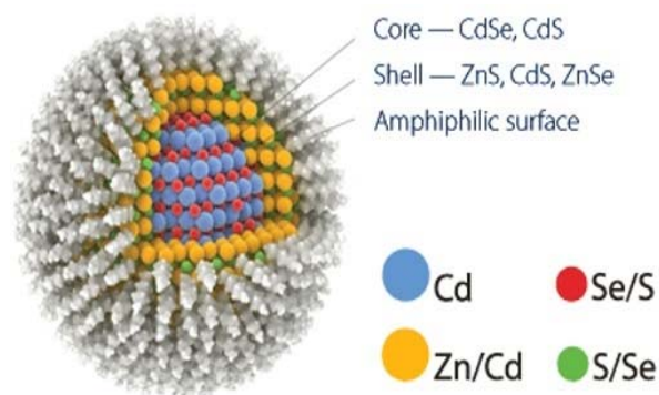
Figure 3. The schematic core-shell configuration of the quantum dot, with a core that typically composed of CdS and CdSe and a shell that typically composed of ZnS, ZnSe, and CdS [38].
