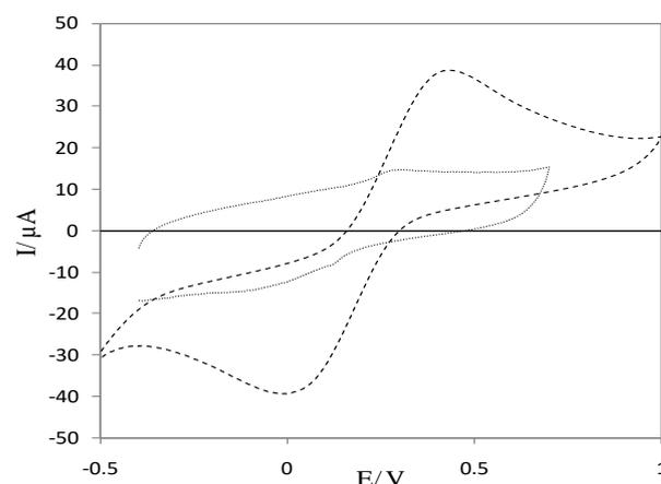
Figure 2. CVs of (—) bare RGr glassy carbon modified electrode, (....) Calcium dobesilate on CNTs glassy carbon modified electrode, (---) Calcium dobesilate on RGr glassy carbon modified electrode in 0.1 M PBS (pH 6.8). The scan rate was 100 mV/s at air-saturated conditions.
