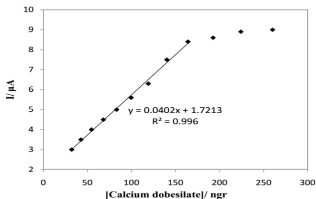
**Figure 4.** Calibration curve for the Calcium dobesilate on RGr glassy carbon modified electrode by chronoamperometry in 0.1 M PBS (pH 6.8) containing various concentrations of Calcium dobesilate at the air-saturated conditions. The Calcium dobesilate concentrations are from 30-270 ng/mL.
