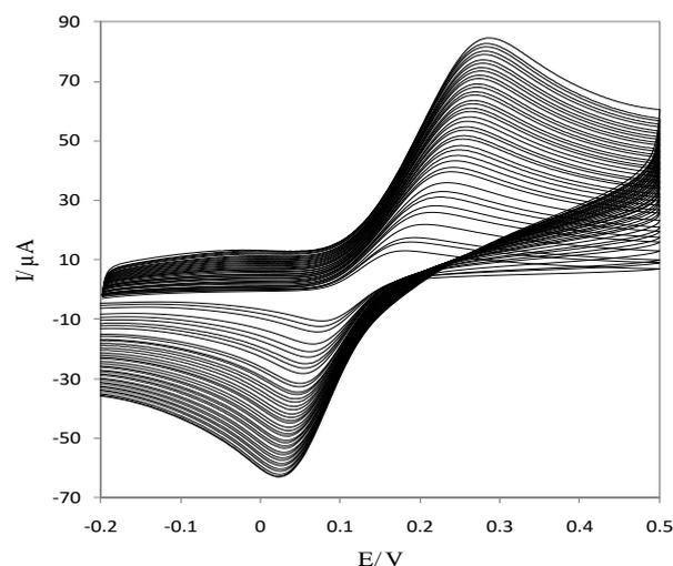
Figure 3. (A) CVs of Calcium dobesilate on RGr glassy carbon modified electrode in 0.1 M PBS (pH 6.8) at various scan rates of 5, 10, 20, 30, 50, 60, 70, 80, 90, 100, 120, 150, 170, 200, 250 and 300 to 1000 mV/s from inner to outer, respectively.
