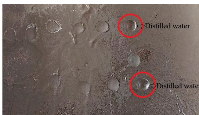
Figure 7. Vials containing fragments of outer membrane proteins were placed on an aluminum plate, and ice nucleation was evaluated using the frozen droplet technique. The LAUDA® Alpha RA 8 Refrigerating Circulator was employed to evaluate ice nucleation activity. At -5 °C, all droplets containing the outer membrane of the Pseudomonas syringae were frozen. Distilled water was used as a negative control, shown in the red circle.
