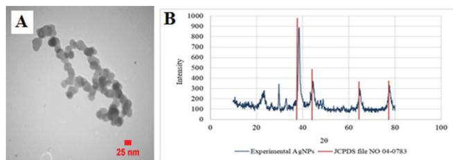
**Figure 1.** TEM image of spherical silver nanoparticles with smooth surfaces (A). Matching the XRD peaks of the tested nanoparticles with the pattern peaks (B).
