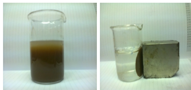
Figure 5. Photograph of magnetic separation for MIP nanoparticles.
