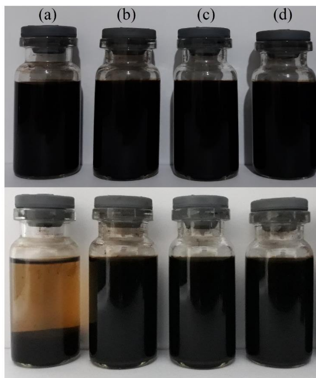
Figure 5. Colloidal Stability of Nanoparticles for (a) the Untreated Sample, (b), (c), and (d) the Samples Treated with 50, 75, and 100W (15 min).
